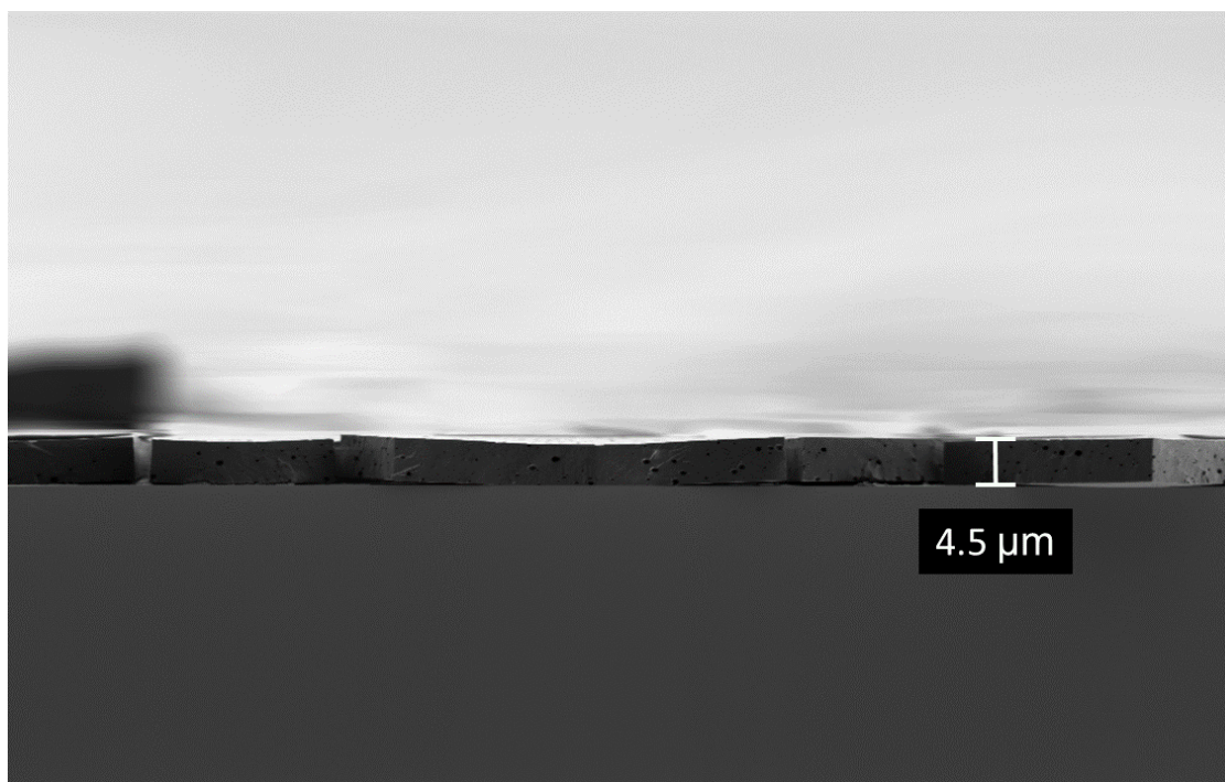
Figure A4.31. SEM of a cross-section of a thin film prepared by drop casting 4.10F-[Co 2 (CO) 6 ] 2 onto a silicon wafer.
